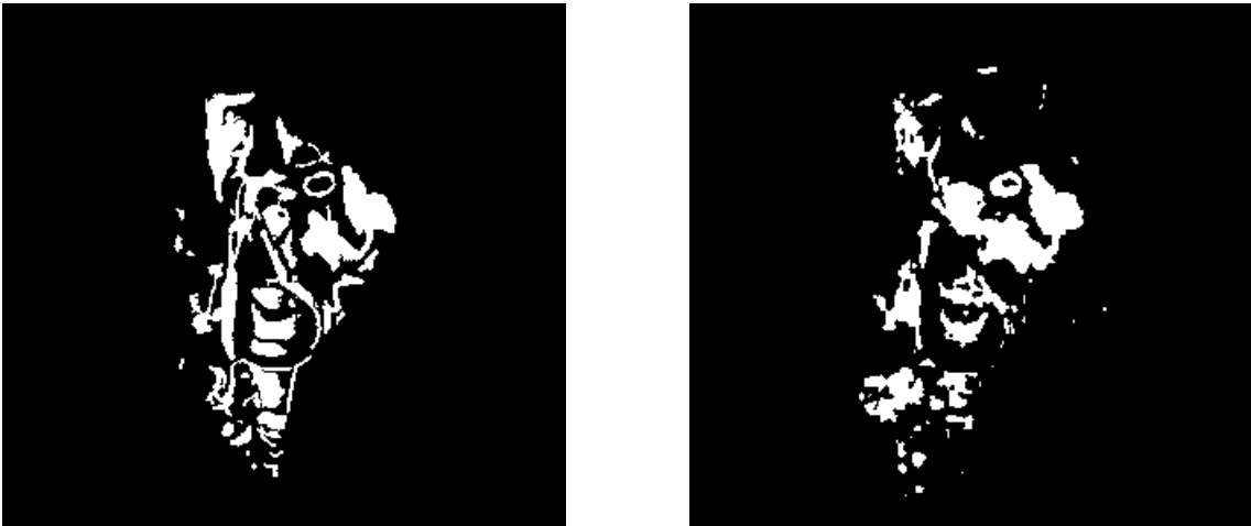
Figure 3.5: A pair of labelled change prediction mask images. Left: ground-truth label; right: change prediction by LSNet.
