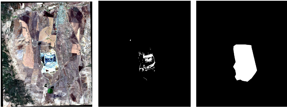
Figure 3.4: From left to right: an RGB Sentinel-2 image tile, the corresponding change mask label, and the area mask polygon.
