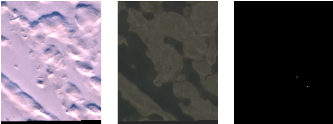
Figure 4.12: Snow-cover seasonal prediction. From left to right: Sentinel-2 'pre' image tile; Sentinel-2 'post' image tile; TinyCD model change predictions.
