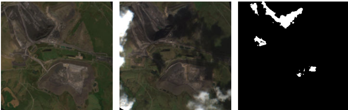
Figure 4.10: Prediction example. From left to right: Sentinel-2 ‘pre’ image tile; Sentinel-2 ‘post’ image tile; LSNet model change predictions.
