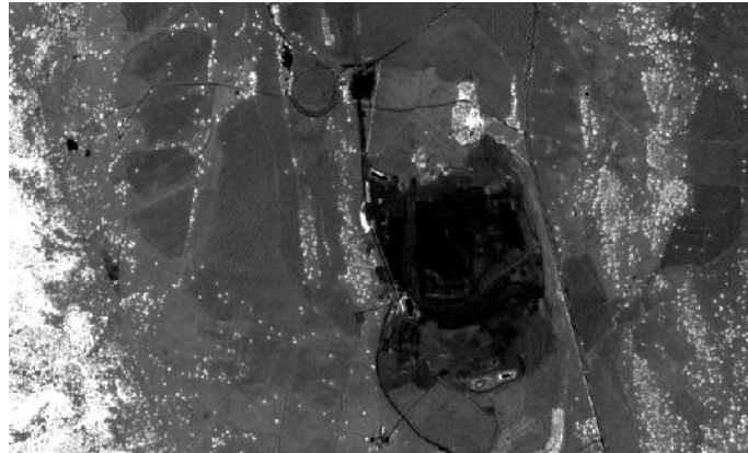
Figure 1.3: Example image demonstrating an NDVI matrix. Pixels which are more white represent a higher NDVI, and vice-versa.
